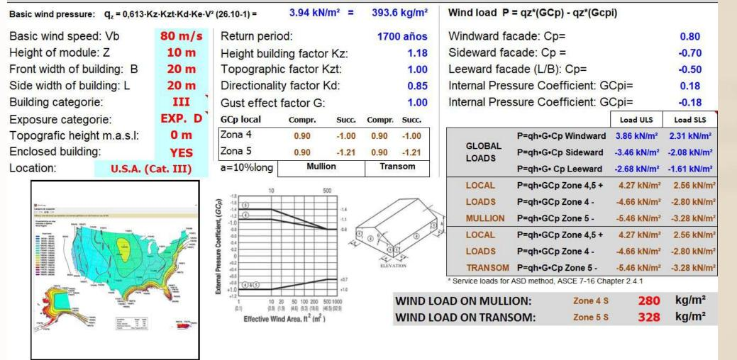
Our window systems are specially manufactured to comply with or exceed ASCE7 16 wind loads.
